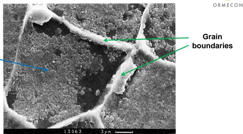
SEM picture of a steel surface treated with the **ORGANIC METAL**. The Fe<sub>2</sub>O<sub>3</sub> layer has started to grow within the grain boundaries.
